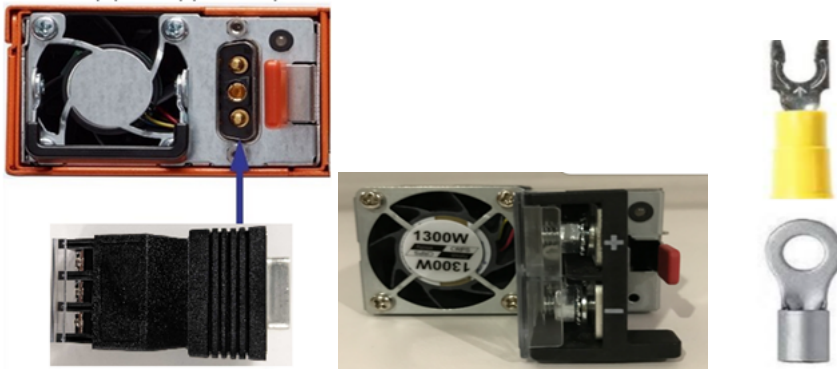
Figure 10 Connecting DC Power Supply Module (2 different type of power modules)
