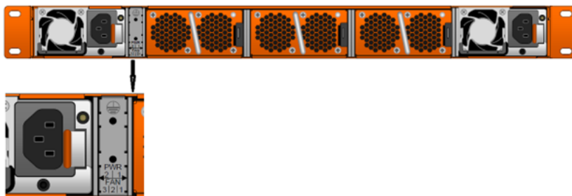
Figure 7 Holes for Ground Screws
